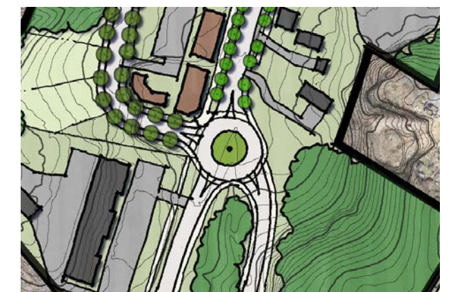
The Illustrative Plan depicts a conceptual design for a roundabout at the intersection of Taft Highway. While the precise location and design requires additional study, the concept illustrates how the roundabout can improve the operation of this key intersection, create an opportunity to connect Timesville Road (and the Town Center) to the intersection, and creates a gateway into Walden with a focal point for art or sculpture in the center. Below is an image of a roundabout in Nashville, TN.
