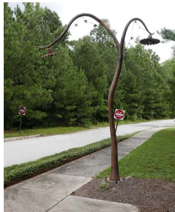
Outdoor lighting has a variety of aesthetics. The key to minimizing light pollution is to choose fixtures with shields that direct light down to the ground or directly on the object.
