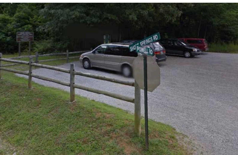
Trail parking areas should be designed to compliment the natural character of their surroundings. Features such as wood rail fences, pervious paving, timber bollards delineating no parking zones, and natural landscaping can formalize parking areas without detracting from the surrounding character.
